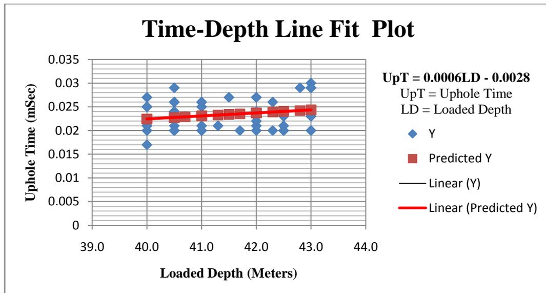
**Fig.21** Uphole time versus loaded depth plot
