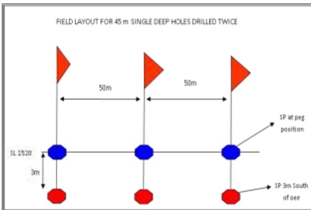
**Fig.13** SDH drilled twice
