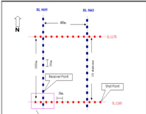
**Fig.2** Receiver and source lines set up
