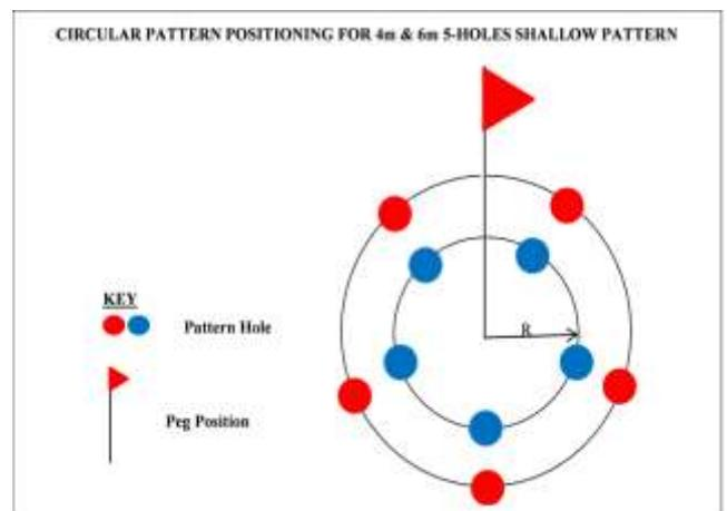
**Fig.16** Circular drill pattern
