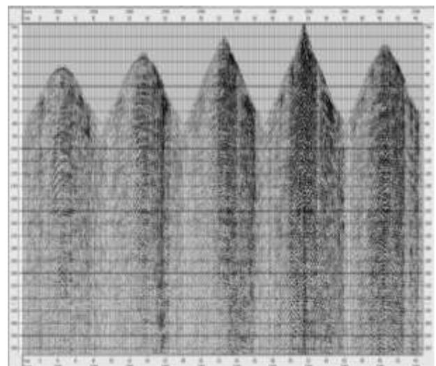
**Fig 20:** Raw shot affecter noise filtration and Attenuation
