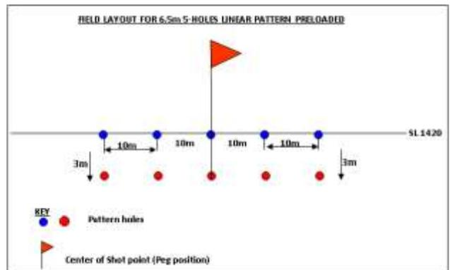
**Fig.15** 6.5m 5-hole linear pattern
