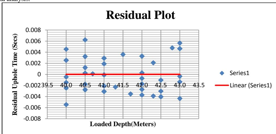
**Fig.22** Plot of residual uphole time versus loaded depth
